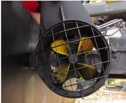
Propeller on Pontoon Undercarriage
